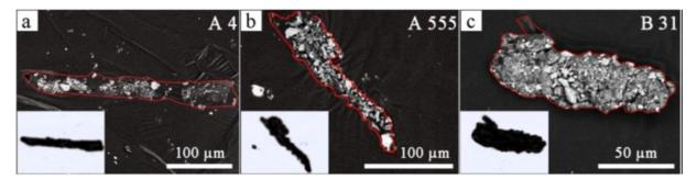
Fig. 1 Scanning Electron Microscopy pictures of typical super-coarse TRWP particles from motorways [10]
